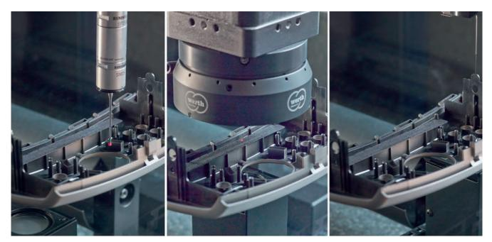
Figure 1. The datum features on a cover are defined using a conventional stylus system, then the flatness is measured with a laser distance sensor, and the flexible tab is measured with a fiber probe. (© Werth)
