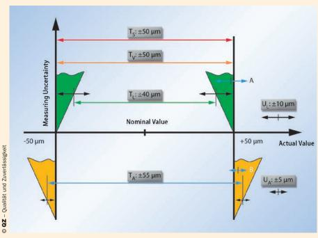
Figure 1. Effect of measurement uncertainty on the residual tolerance for shipment approval and receiving acceptance:  $T_{\rm S}$  Specified drawing tolerance,  $U_{\rm L}$  Uncertainty of the supplier's measuring machine,  $T_{\rm L}$  Tolerance for release for shipment,  $U_{\rm A}$  Uncertainty of the measuring machine at receiving,  $T_{\rm A}$  Tolerance for release of incoming goods
