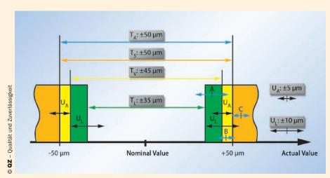
Figure 2. Contractual tolerances ensure that the contractual conditions are unambiguous:  $T_{\rm S}$  Drawing tolerance,  $U_{\rm A}$  Uncertainty of the measuring machine upon receipt by the customer,  $T_{\rm V}$  Contractual tolerance,  $U_{\rm L}$  Uncertainty of the supplier's measuring machine,  $T_{\rm L}$  Tolerance for release for shipment.
