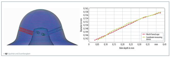
Fig. 2. Comparison measurement of the diameter of a fuel injection nozzle with computed tomography and high-precision fiber probe (a); display of measured volume and measuring point cloud in the area of the spray . (© Werth Messtechnik)
