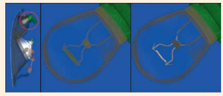
Figure 2. Voxel volumes of a car headlight: tomography at low resolution (left), partial view (middle), and high-resolution region-of-interest tomography of the luminous element (right)
