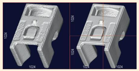
Figure 1. Point clouds (STL view) measured using tomography at low resolution (left) and using raster tomography at high resolution (right)
