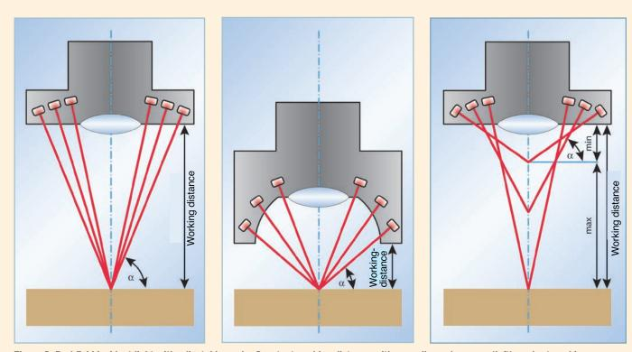
Figure 2. Darkfield incident light with adjustable angle: Constant working distance with a small angular range (left) or short working distance with a medium angular range (center) and MultiRing with a variable working distance and large angular range (right)
