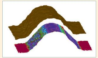
Figure 1. High-resolution area measurement with 3D Patch: Meshed view of the measured surface (top), color-coded deviation plot to the CAD model (bottom)
