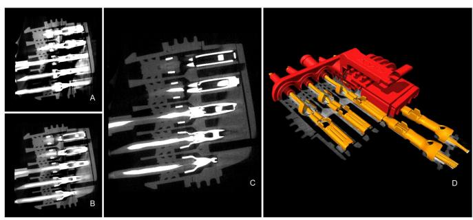
Werth Multi-Spectra-Tomography: by combining several CT measurements (A and B) tuned to each specific material, artifacts are minimized (C and D)
