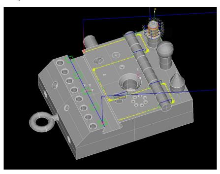
Scan path and point distribution on a CAD model
