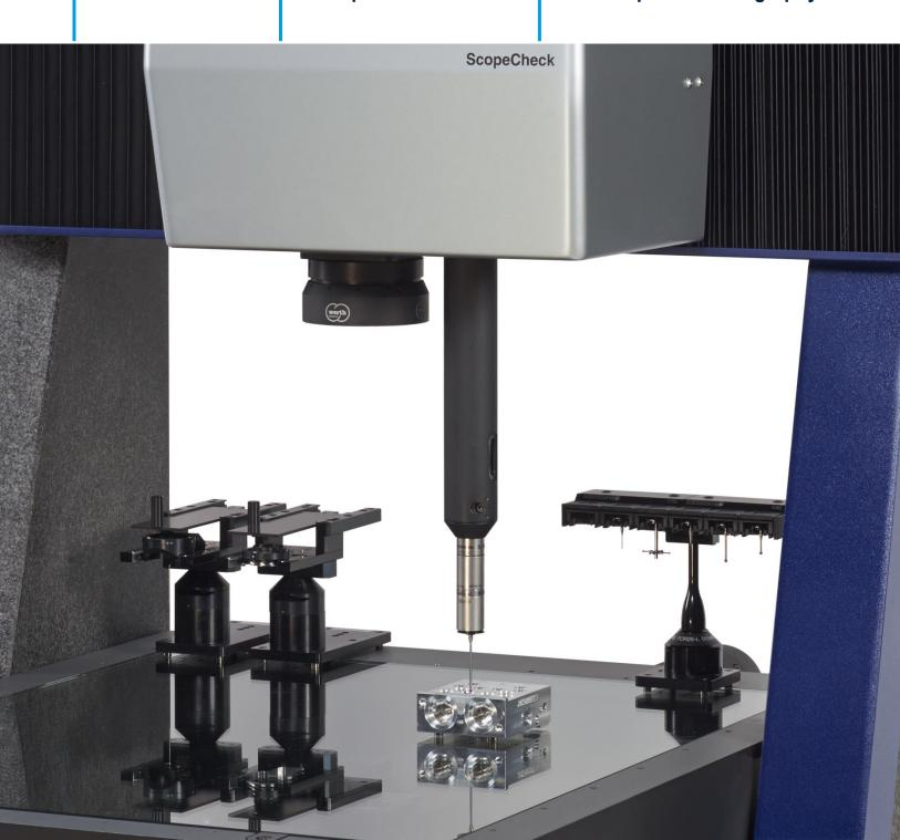
ScopeCheck® FB DZ – collision-free measurements also on the shop floor: dual ram approach for optimal measuring with each sensor, for example image processing sensor or touch probe (cover picture)
