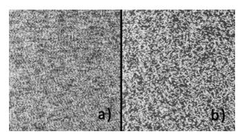
The orientation of the glass fibers – which are just a few micrometers thin – in the fiber reinforced plastic workpiece become clearly visible only during measurement using drift correction (b)
