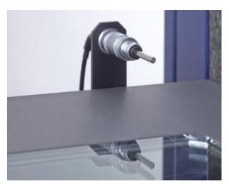
Temperature sensor in the measurement range
