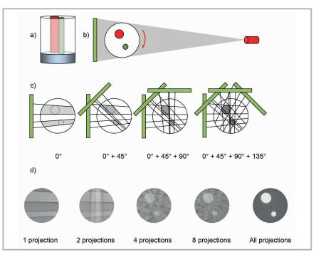
Fig. 1 Calculating volume data by back projection of the filtered radiographic images: a) Object, b) X-ray beam path in one section plane, c) Principle of stepwise back projection and superimposing, d) Result of reconstruction with different numbers of back projections for a real workpiece. (© Werth)
