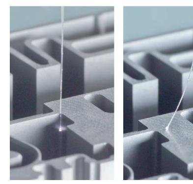
Figure 2. Even if there is an error in positioning, the probe will not be destroyed: left: contact procedure; right: positioning error.
