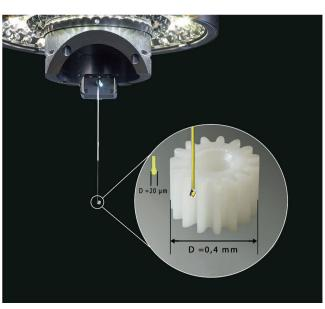
Figure 1: Measurement of a micro gear with the Werth Fiber Probe – the fiber is guided in a metal tube. (© Werth) touch trigger probes is that the coordinate measuring machine is brought into contact with the measuring object to determine a measuring point, and then has to be moved out of contact again.
