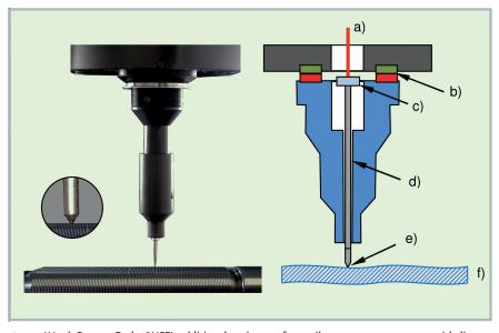
Figure 2. Werth Contour Probe (WCP): additional equipment for tactile contour measurement with distance sensors: a) Measurement beam, b) Magnetic interface, c) Mirror, d) Guide, e) Probe tip, f) Workpiece (© Werth)
